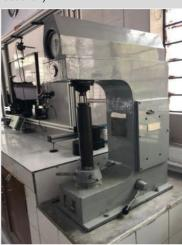
Hardness Testing Apparatus
