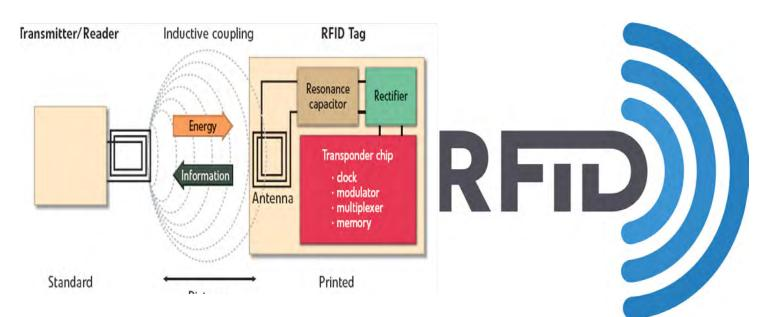
to be checked individually thus making process time consuming. Tags of different types can be physically removed with a special tool or deactivated electronically once items have been paid for. On leaving the shop customers have to pass near an RFID detector; if they have items with active RFID tags, an alarm sounds, both indicating an unpaid-for item, and identifying what it is.
