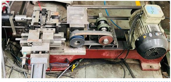
Fig. 3: Linear Friction Welding Setup
