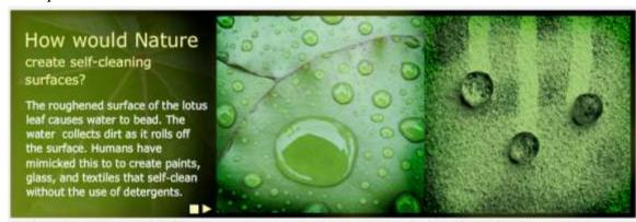
Creating self cleaning surfaces inspired by the lotus leaf. Paints and surface treatments that self clean in the rain. The tiny texture on the surface allows the water to bead and drag away any dirt.
