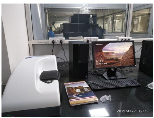
TG-DTA/DSC (Setaram Instrumentation, France, LABSYS EVO 1150°C, DSC131 EVO analyser)
