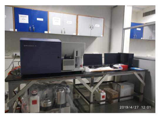
Stopped-Flow Reaction Analyzer, Double mixing system with Abs and Fluorescence detection
