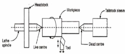
Working principle of lathe machine
