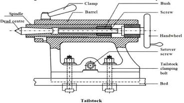
**Bed:** The bed is a heavy casting in which working parts of the table are mounted. It carries the head stock and tail stock for supporting the workpiece and provides a base for the movement of carriage assembly which carries the tools.
