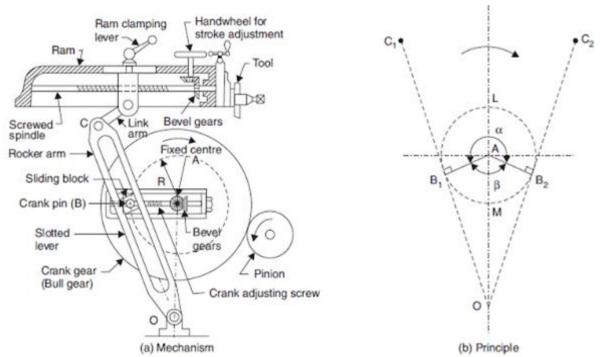
Quick return mechanism of a shaper machine
