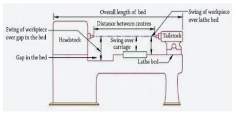
Specification of a lathe machine
