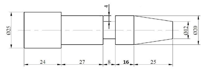
**Object:** To study and perform various operations on a given mild steel job by a lathe machine.
