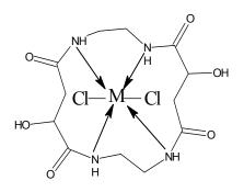
Proposed octahedral structure of metal complexes [M= Co(II), Ni(II),Cu(II)]
