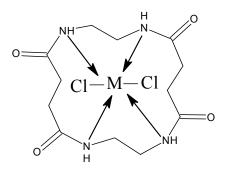
Proposed octahedral structure of metal complexes [M= Co(II), Ni(II), Cu(II)]
