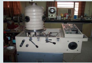
Thermal Evaporation System
