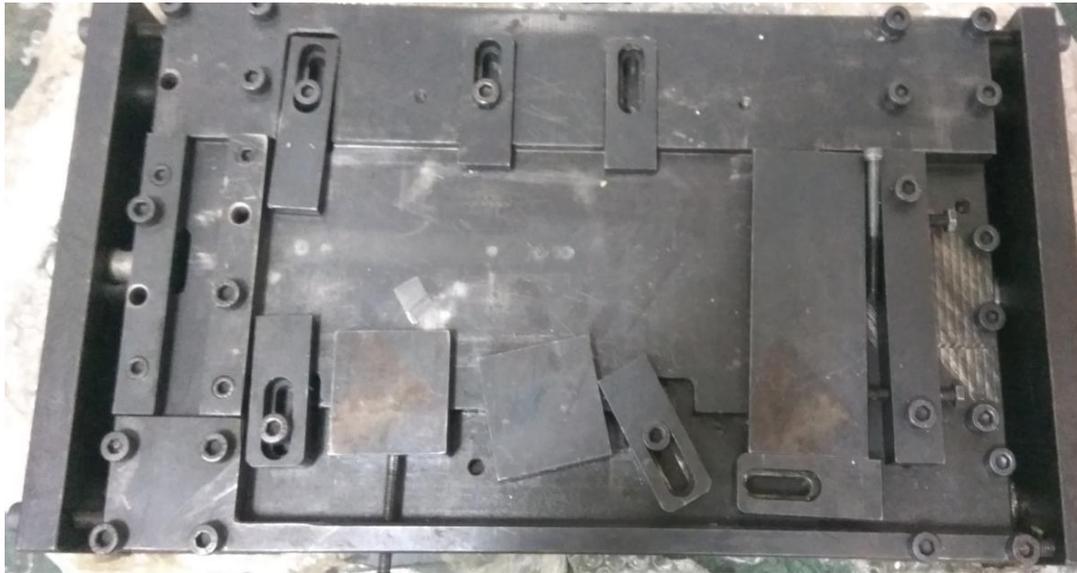
**Fig. 1: Friction Stir Welding Fixture**
