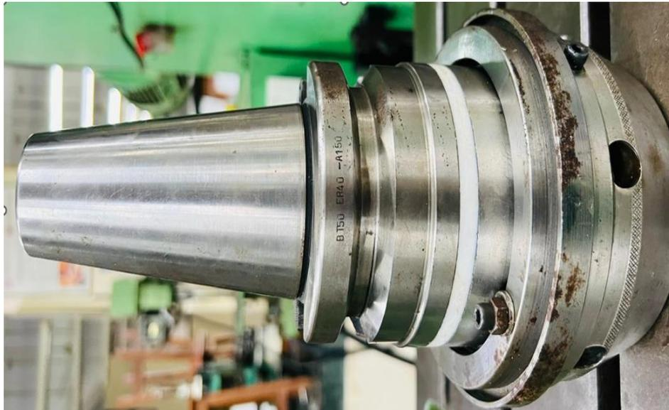
Fig. 2: Tool Holder/Adapter
