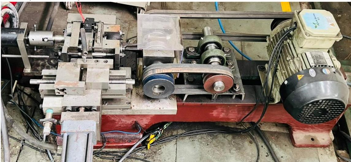
Fig. 3: Linear Friction Welding Setup
