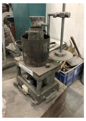
VEE BEE TESTING APPARATUS
