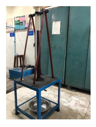
FALLING SPHERE VISCOMETER
