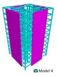
EFFECT OF DIFFERENT POSITIONS OF SHEAR WALL IN A BUILDING
