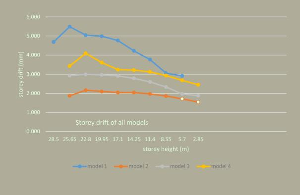
Maximum storey drift permitted = 0.004 × storey height(m) = 0.004 × 2.83 = 0.0032m = 11.32 mm
