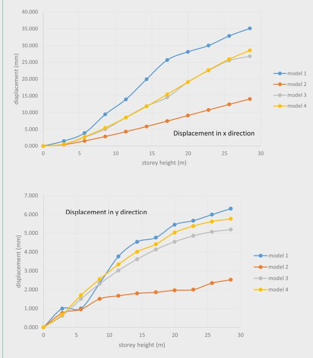
The above illustration shows the displacement in the x and y direction. It has been observed that model (1) that is without shear wall has maximum displacement in both directions. However, model (2) shows the minimum displacement in both directions.
