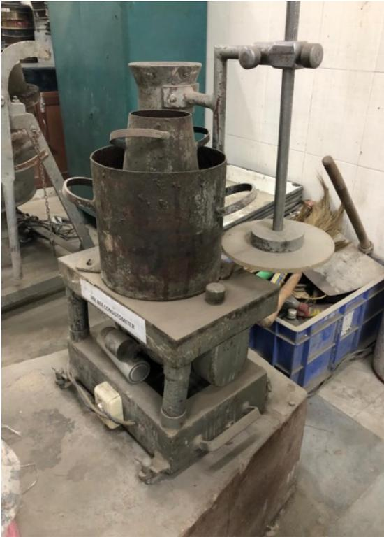
VEE BEE TESTING APPARATUS
