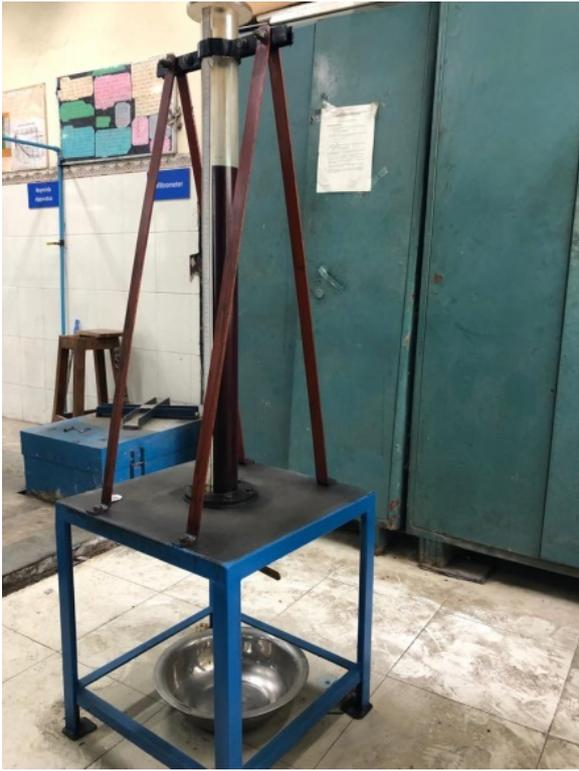
FALLING SPHERE VISCOMETER
